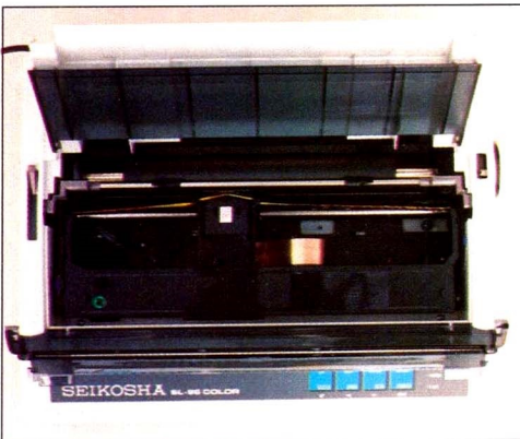
A view into the printer, showing the colour ribbon cartridge in place. The front panel controls are simple to use
